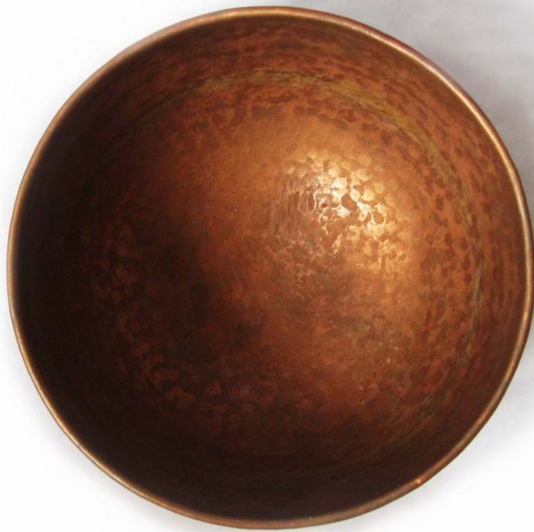
Bowl, copper, technique: hammer. diameter: 16 cm, hight: 8 cm
